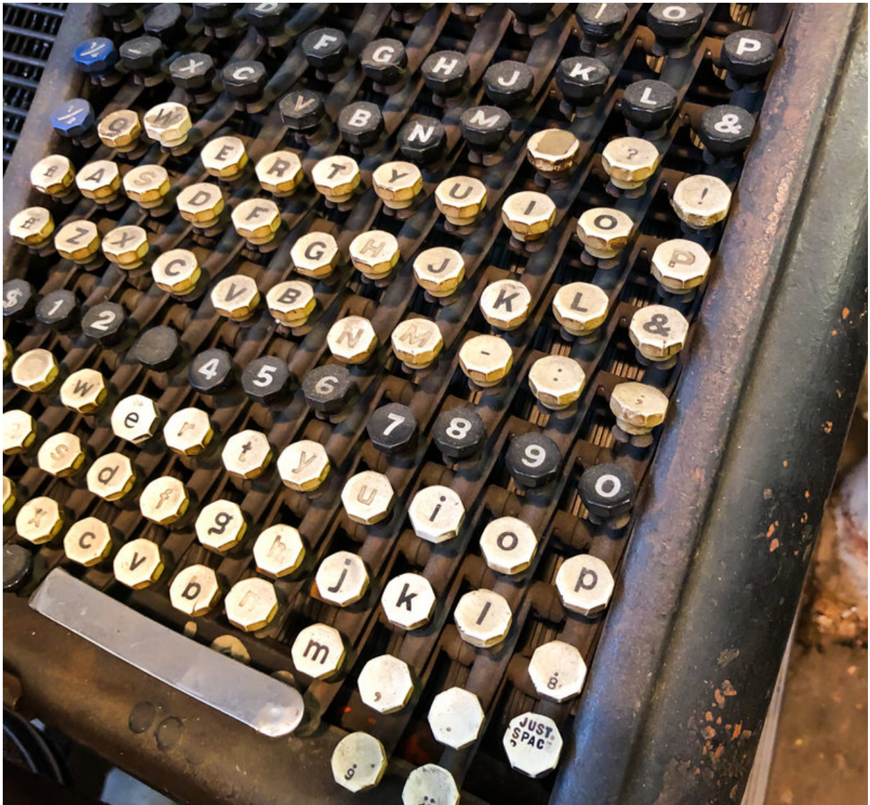
A Monotype keyboard features a familiar QWERTY layout, but with separate keys for upper and lower case.
