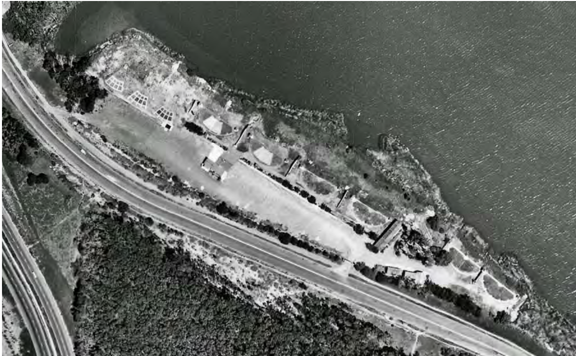
Historic Image 15. Aerial view in 1958. Changes since 1955 aerial (Historic Image 14) include addition of concrete trap yardage marker pavement to the interior of Fields 4 and 5 that allowed these fields to be used for both skeet and trap. Source: Pacific Aerial Surveys.
