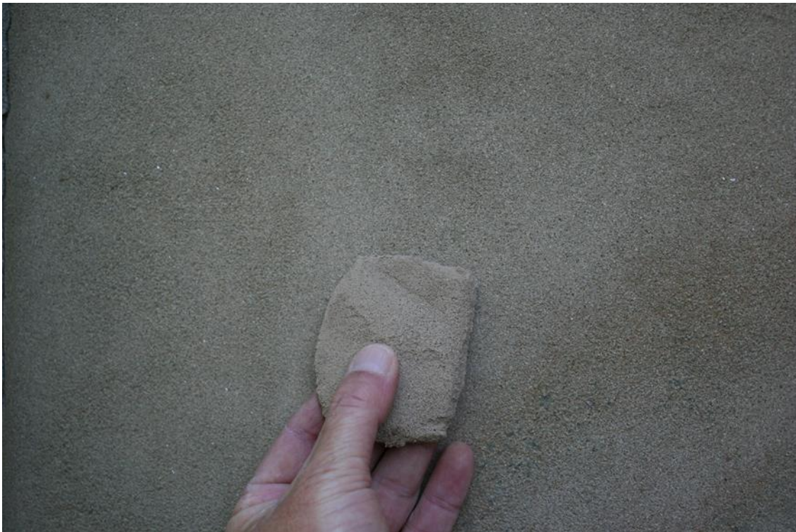
Image 7. Color match at ashlar masonry with mortar sample TM-265A in shade.
