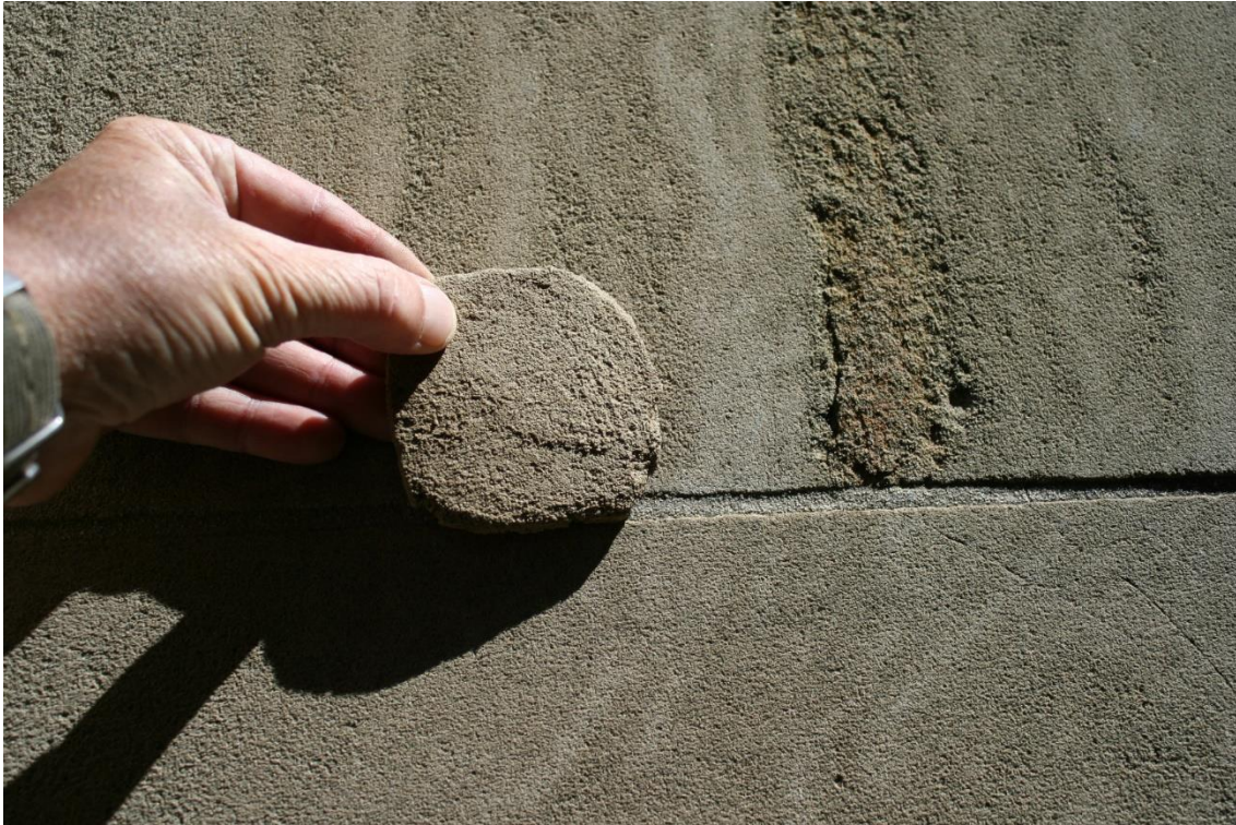
Image 6. Color match at ashlar masonry with mortar sample TM-265A in sunlight.
