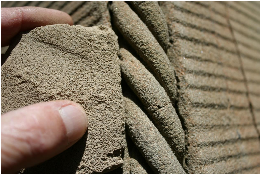
Image 9. Color match at decorative element with mortar sample TM-273C in sunlight.
