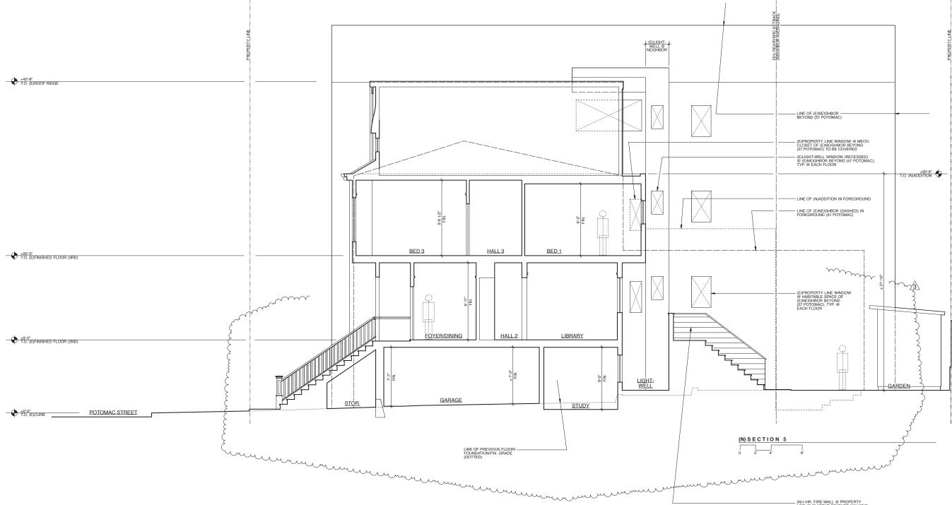
. (N)1-HR. FIRE-WALL @ PROPERTY LINE (3'-6" ABOVE FINISHED WALKING SURFACE) W/(N)WOOD SIDING, PAINTED
