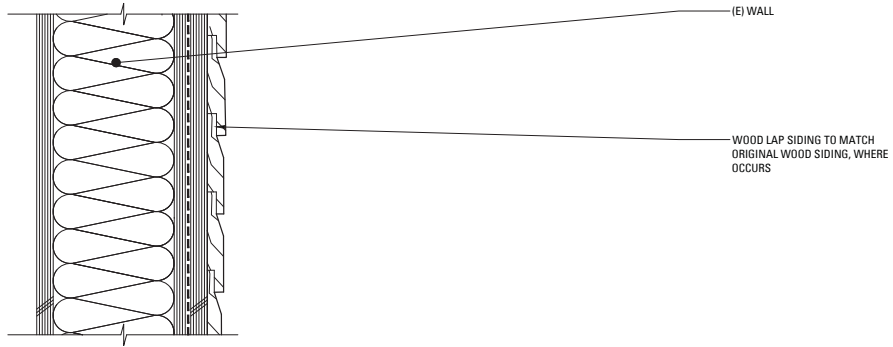
7 WALL SIDING DETAIL SCALE: 3" = 1'-0"
