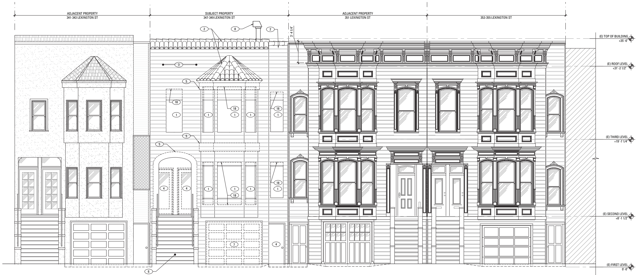
1 FRONT ELEVATION - CURRENT CONDITIONS SCALE: 1/4" = 1'-0"
