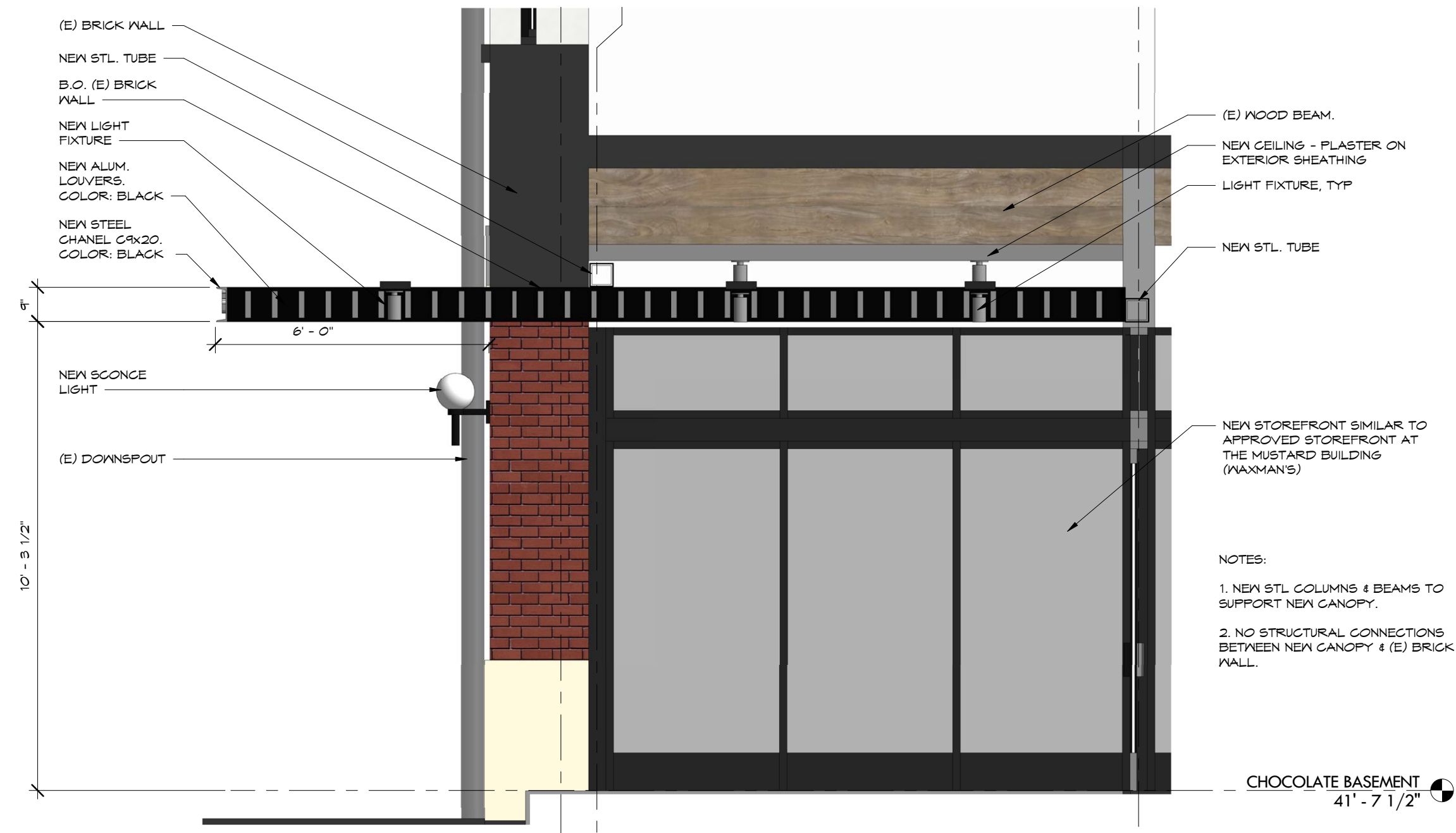
Building section (Scale: 3/8" = 1'-0")
