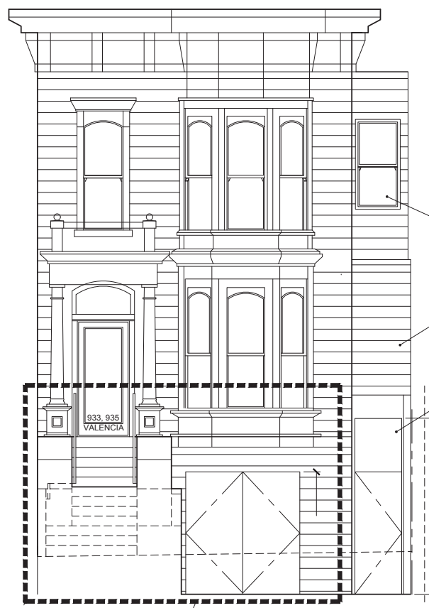
4 PROPOSED WEST ELEVATION (FRONT) SCALE: 1/4"=1'-0"
