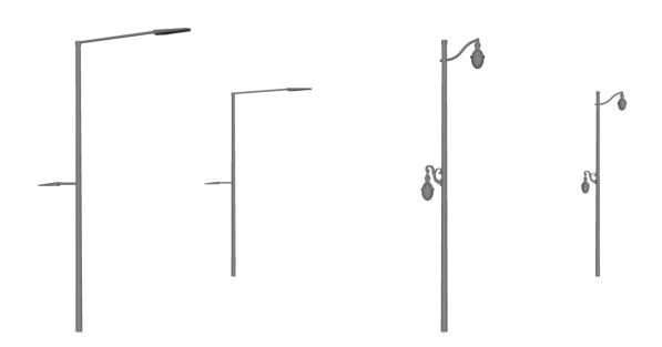
Left: OCS pole as approved. Right: Alternative OCS pole with replica pedestrian and street lamps and brackets.
