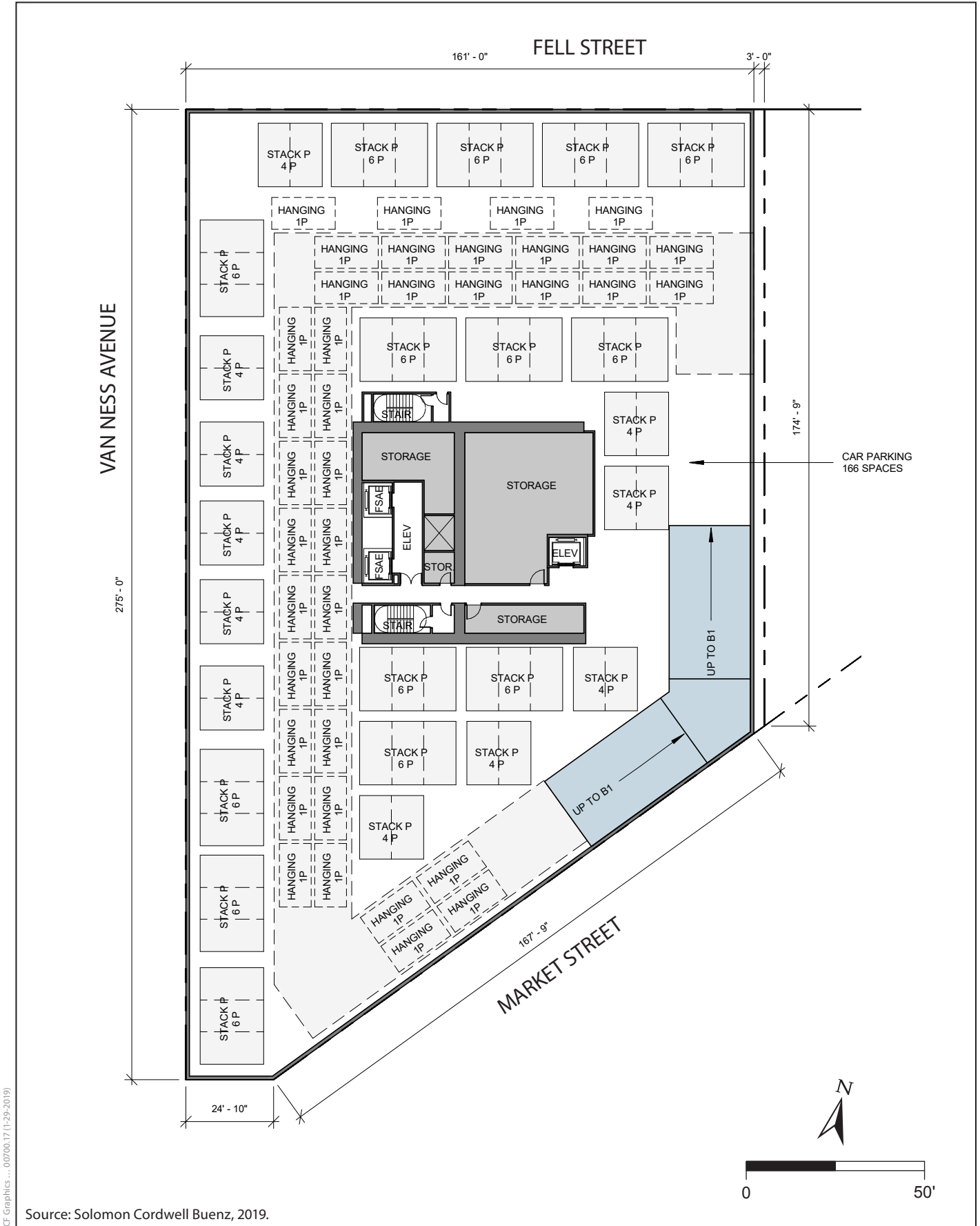
Figure 2-22 30 Van Ness Avenue Project – Proposed Basement Level 2 Plan
