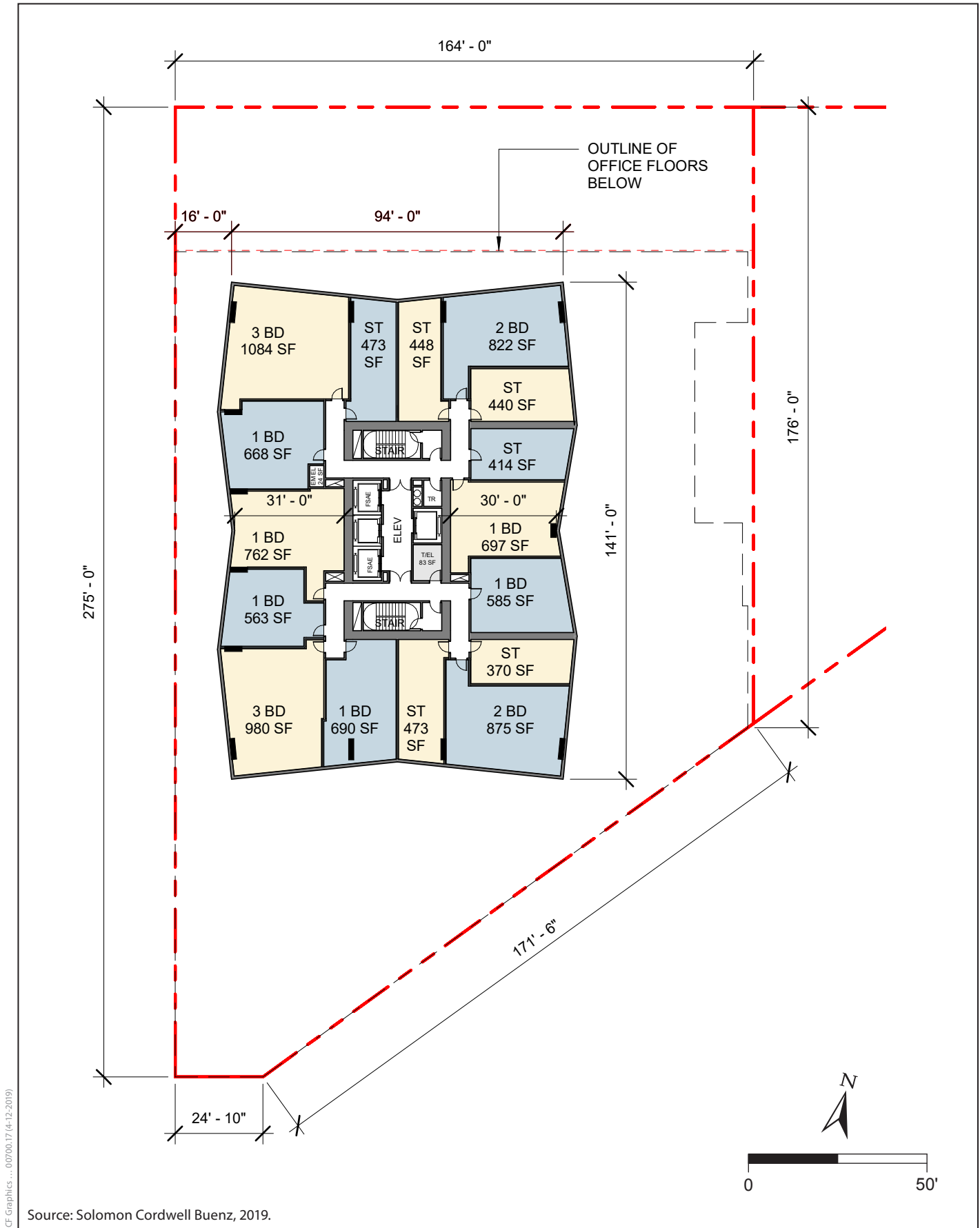
Figure 2-26 30 Van Ness Avenue Project – Proposed Floor Plan Typical of Floor 14 through 47
