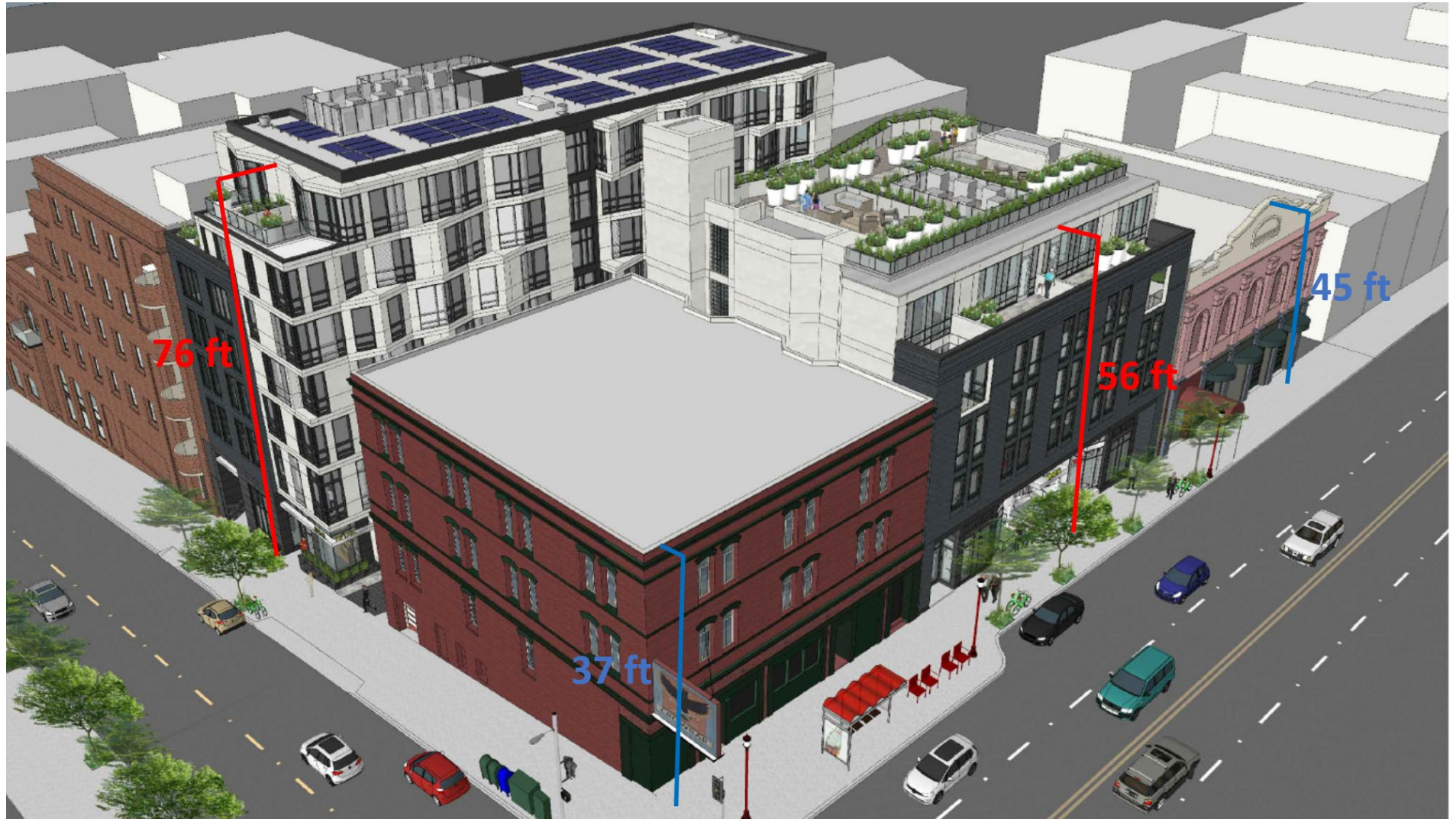
Figure 4. Physical height above Montgomery and Broadway for two proposed buildings at 425 Broadway (Montgomery building = 76 feet, Broadway building = 56 feet)
