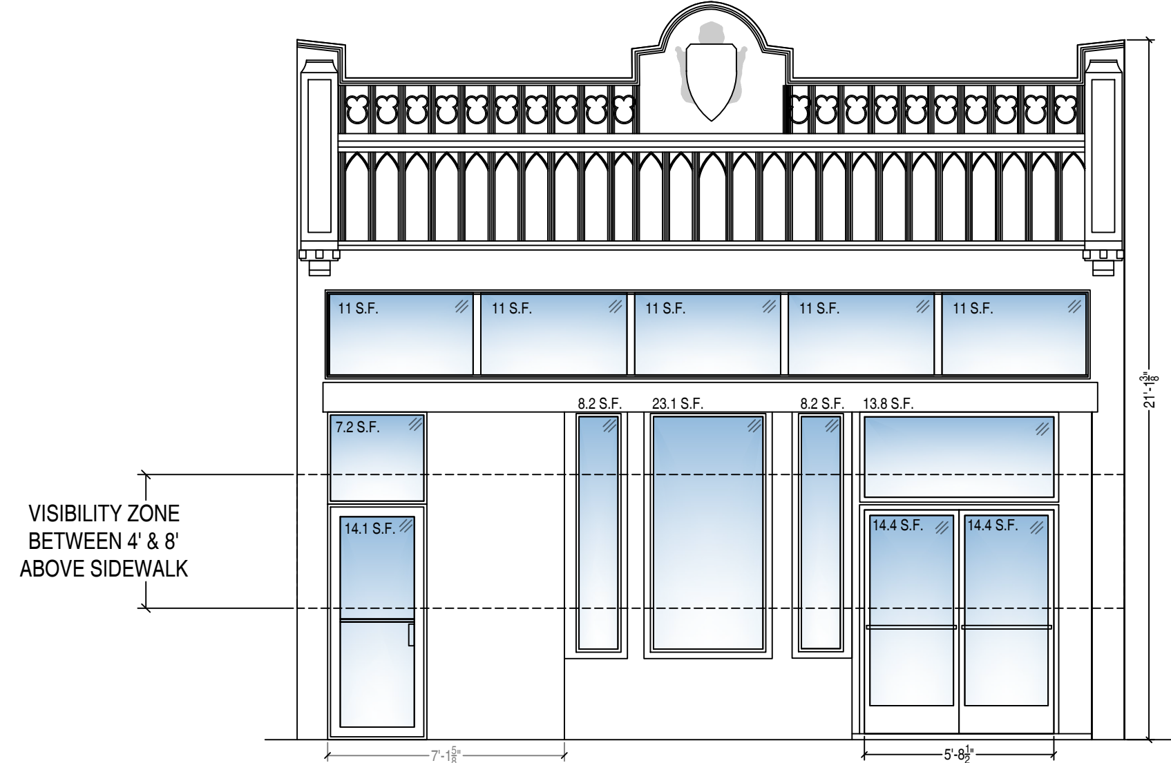
(E) STORE FRONT SIGNAGE ELEVATION (WEST) SCALE: 1/4" = 1'-0"
