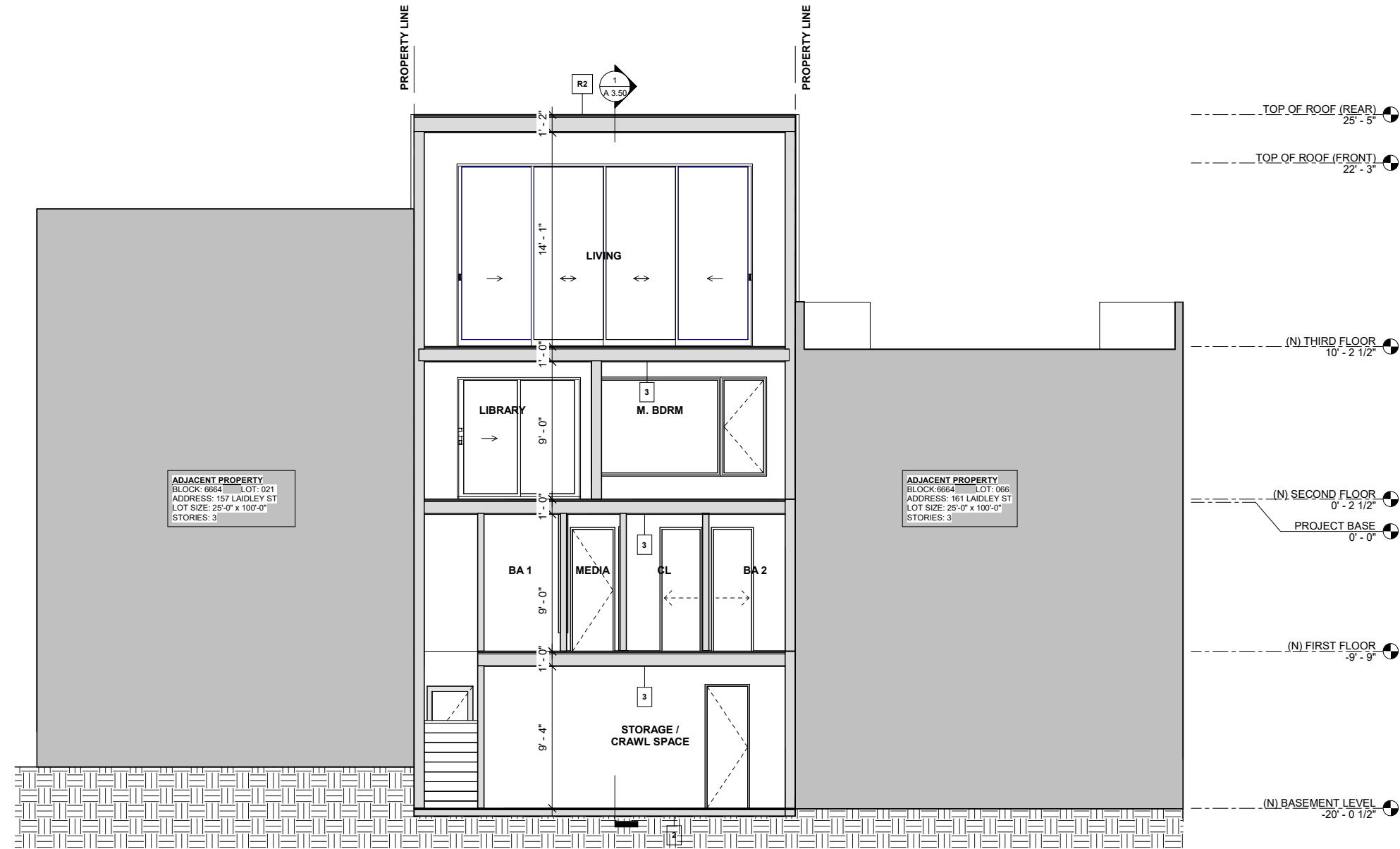
1 PROPOSED TRANSVERSE SECTION 1/4" = 1'-0"
