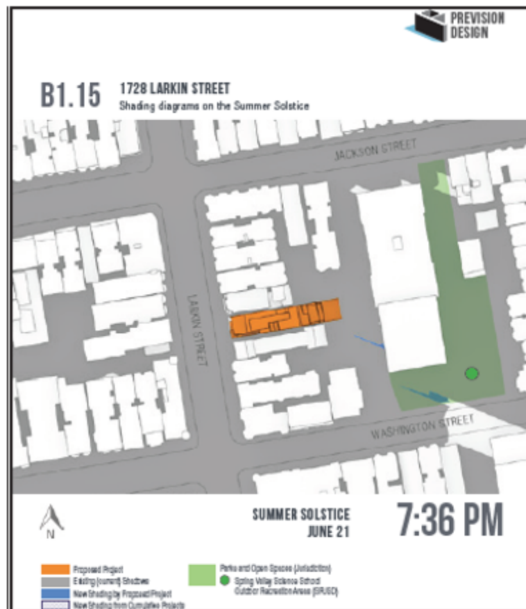
Dark grey depicts shadow cast by existing structures; blue depicts net new shadow cast by the Project.
