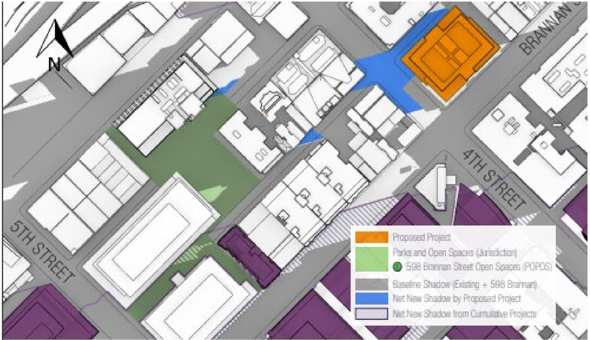
Figure 11: Approximate Largest Area of Net New Shadow on the Future 598 Brannan Street Park (June 21st at 7:30 am)
