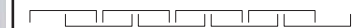
MID-POINT TO MID-POINT INTERLOCKING SEAM PROVIDE 6.5" CADENCE SIMILAR TO WOOD LAP SIDING PATTERNS
