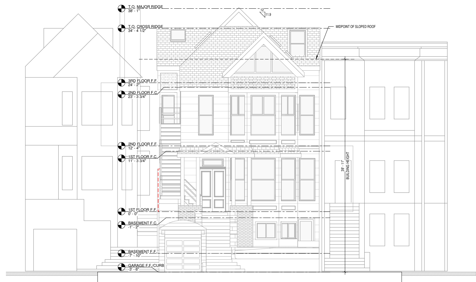
EXISTING SOUTH ELEVATION ① 3/16" = 1'-0"
