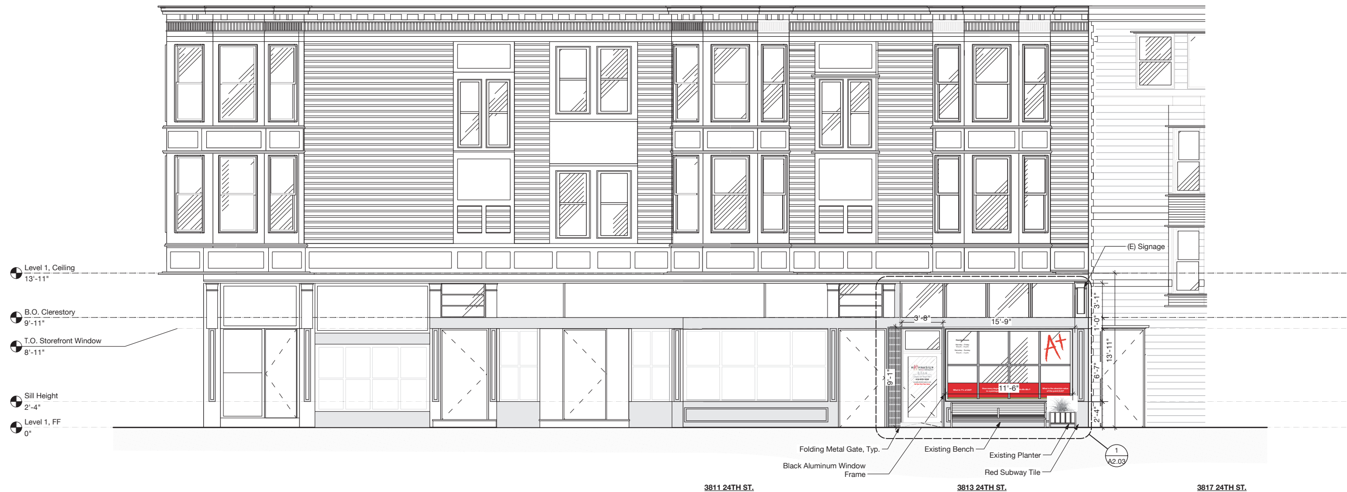
1 North/Front Elevation - Proposed Scale: 1/4" = 1'-0"
