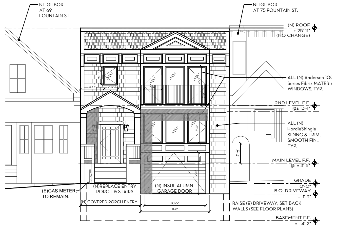
PROPOSED FRONT / WEST EXTERIOR ELEVATIONS 2 ALL NON-REFLECTIVE GLAZING TO BE RECESSED 4" FROM F.O. BUILDING, SEE 3/P2.2 FOR TYP. DETAIL. 1/8" = 1'-0"
