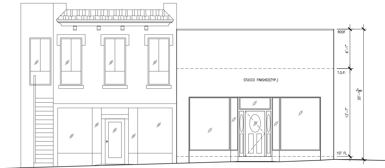
2 EXISTING FRONT ELEVATION (TO BE DEMO) Scale: 1/4" = 1'-0"
