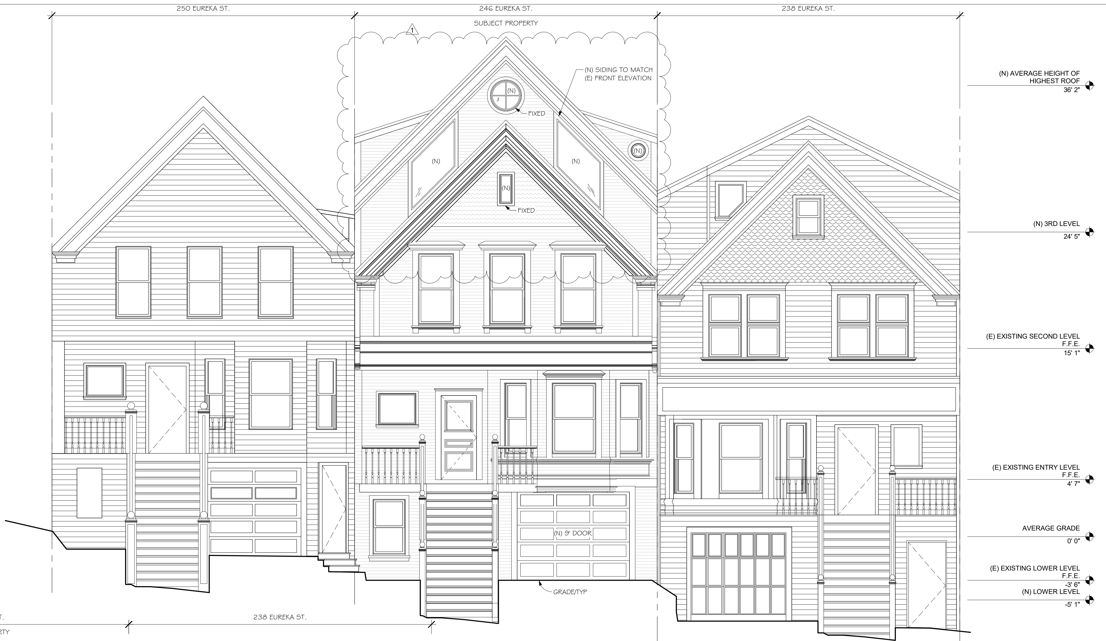
2 EAST ELEVATION - PROPOSED 1/4" = 1'-0"
