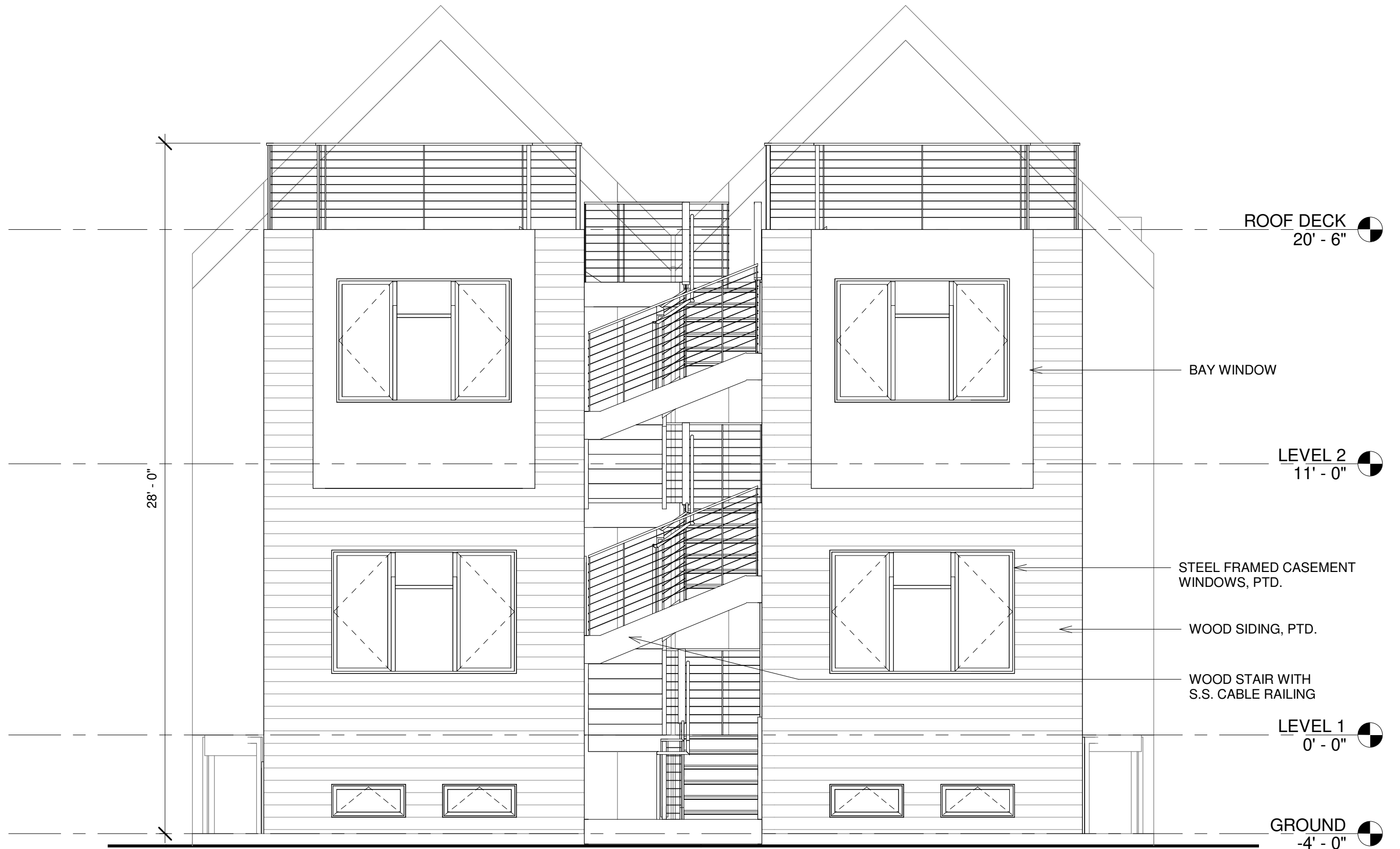
1 PROPOSED REAR ELEVATION 1/4" = 1'-0"
