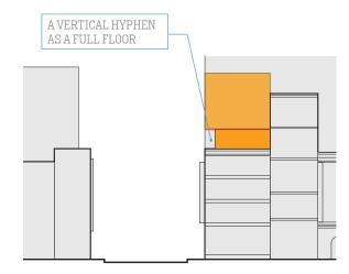
Indent or setback new floors that sit above retained elements to highlight the change in structure, space, and age of new construction. 18 Special topic design guidelines
