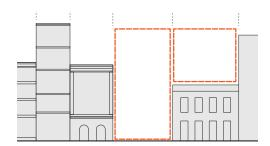
Analyze: Diagram the existing and potential streetwall to find ways to express similar widths and heights.
