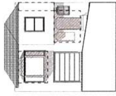
DEMO 13.50' FT REMAN 88.50' FT 2 SOUTH ELEVATION SCALE 1/8" = 1'-0"
