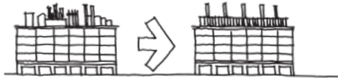
Fig. 45 Screen Mechanical Equipment
