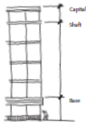
Fig. 47 Base, Shaft, Capital - A Typical San Francisco Building Pattern
