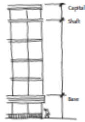
Fig. 56 Base, Shaft, Capital - A Typical San Francisco Building Pattern
