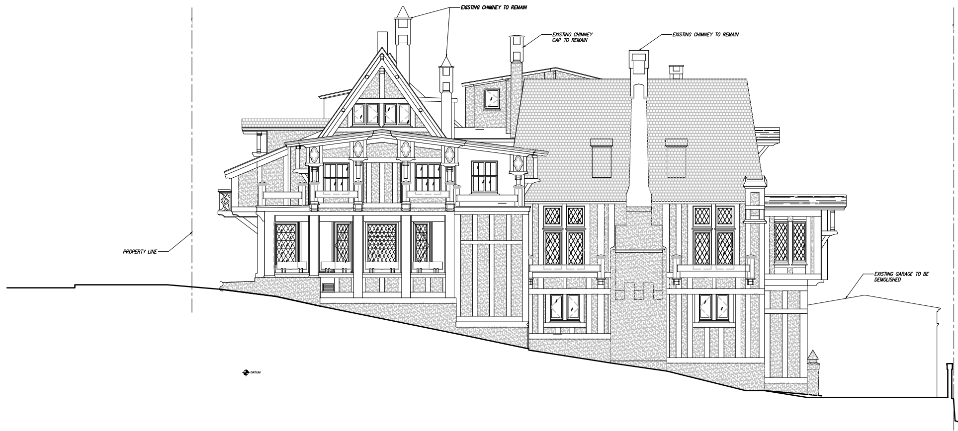
2 EAST ELEVATION - EXISTING SCALE: 1/16" = 1'-0"
