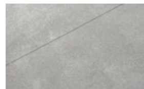
CIP Concrete: Natural Gray w/ Silica Carbide and Water Jet Finish
