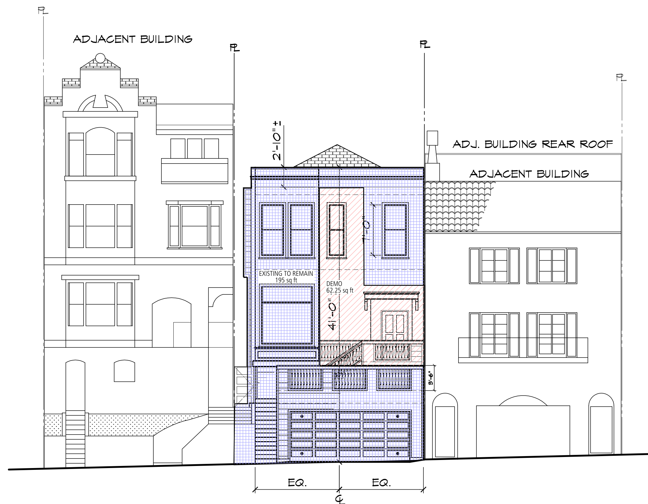
(E) FRONT ELEVATION (NORTH) SCALE: 1/8" = 1'-0"
