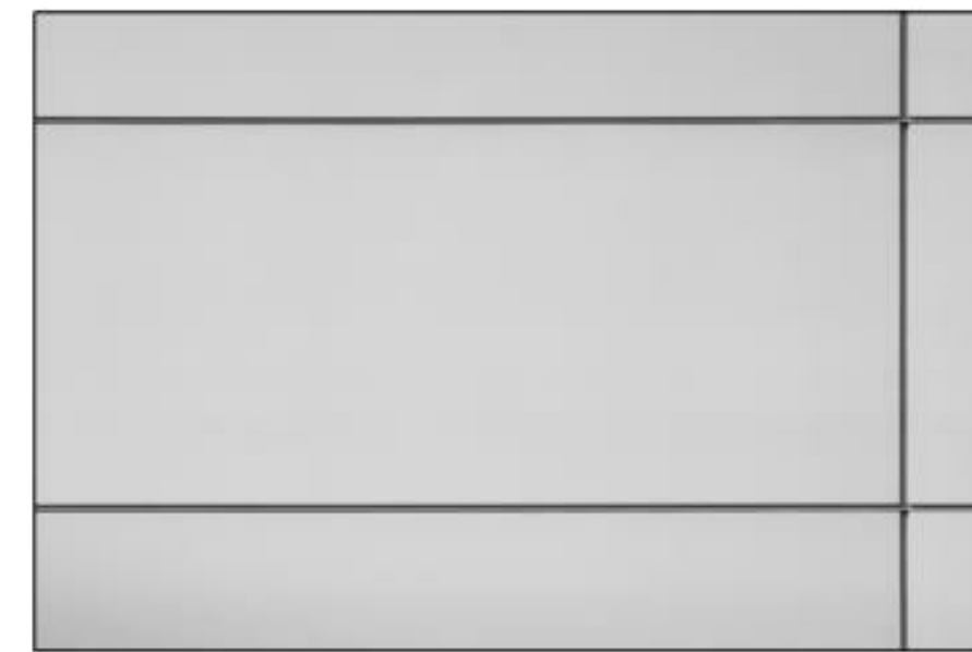
FIBER CEMENT PANEL SIDING ⑤
