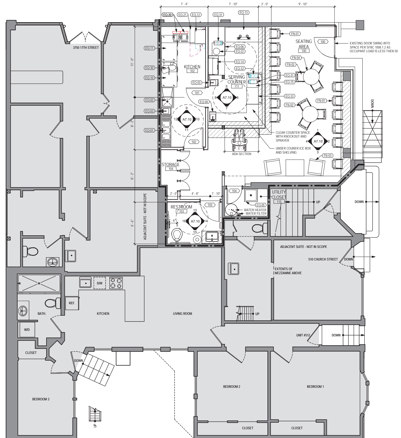
1 PARTITION PLAN - FLOOR 1 SCALE: 1/4" = 1'-0"
