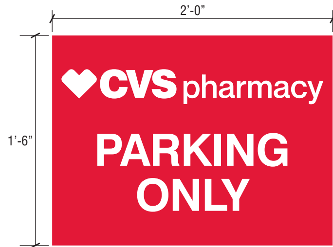
D1-D5 SIGN ELEVATION / PARKING ONLY PANEL QUANTITY: FIVE (5) UNITS REQUIRED SCALE: 1 1/2" = 1'-0"
