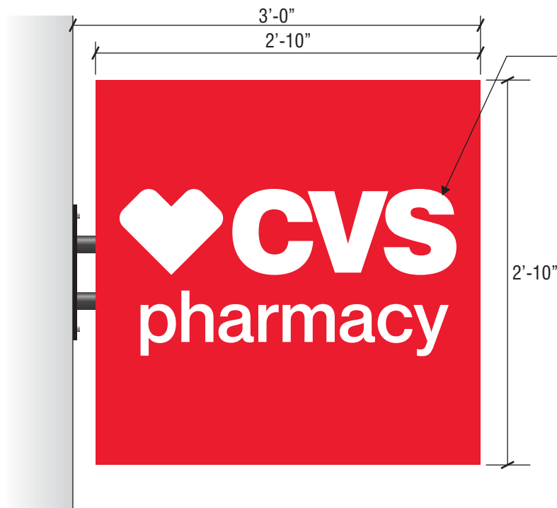
B1 FACE LIT BLADE SIGN WITH ROUTED PUSH-THRU COPY SQ.FT. = 8.02 EACH B2 QUANTITY: TWO (2) SIGNS REQUIRED SCALE: 1" = 1'-0"
