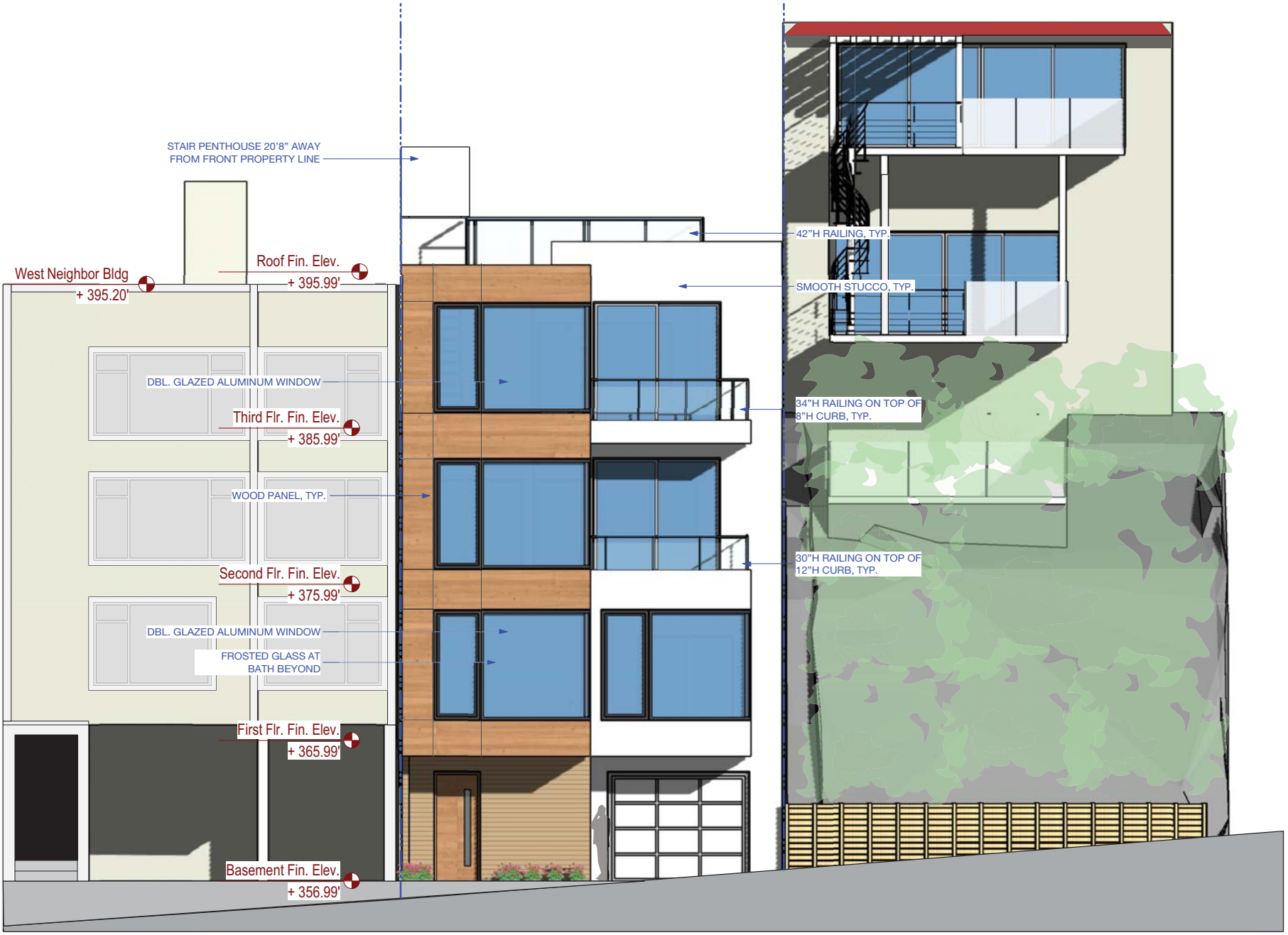
Proposed (South) Facade Elevation 1/4" = 1'-0"
