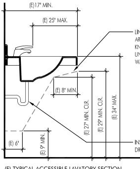
LINE INDICATES MIN. AREA REQUIRED FOR KNEE CLEARANCE UNDER COUNTER OR WALL HUNG LAVATORY
