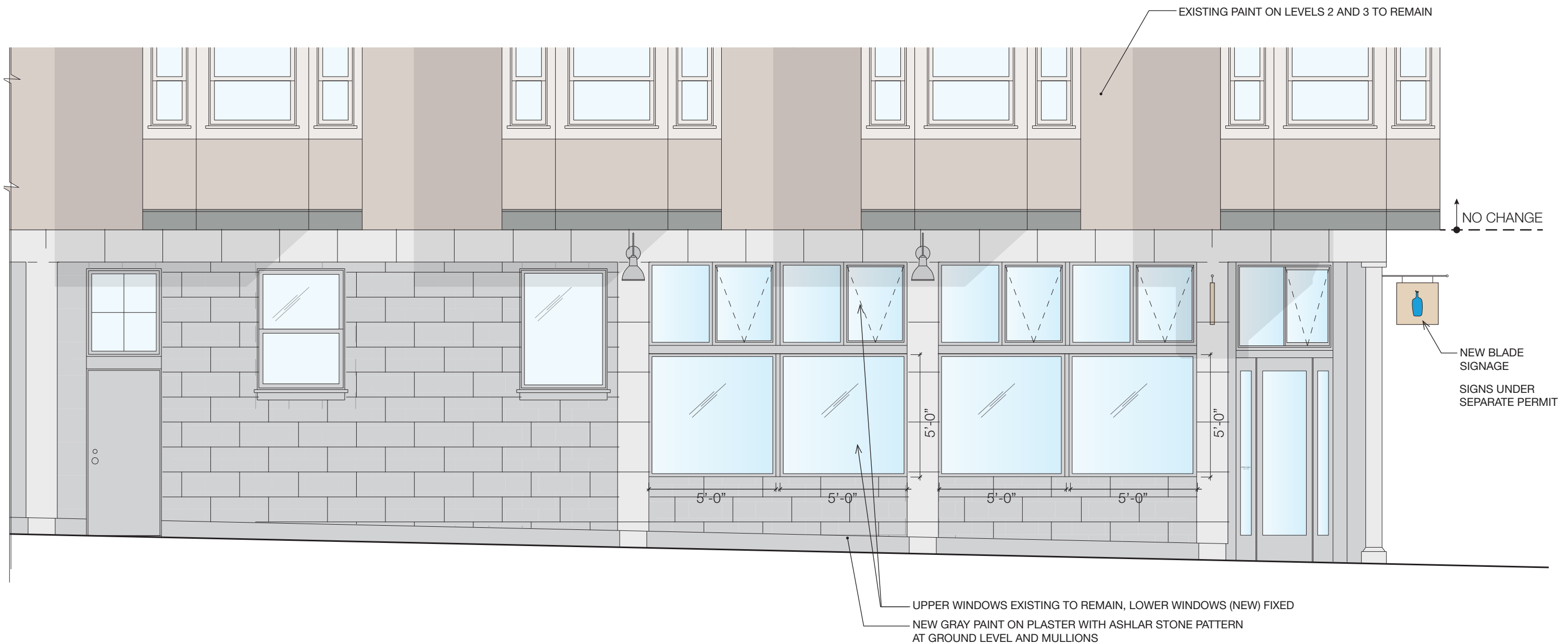
PROPOSED EXTERIOR ELEVATION - SOUTH 1/4" = 1'-0"
