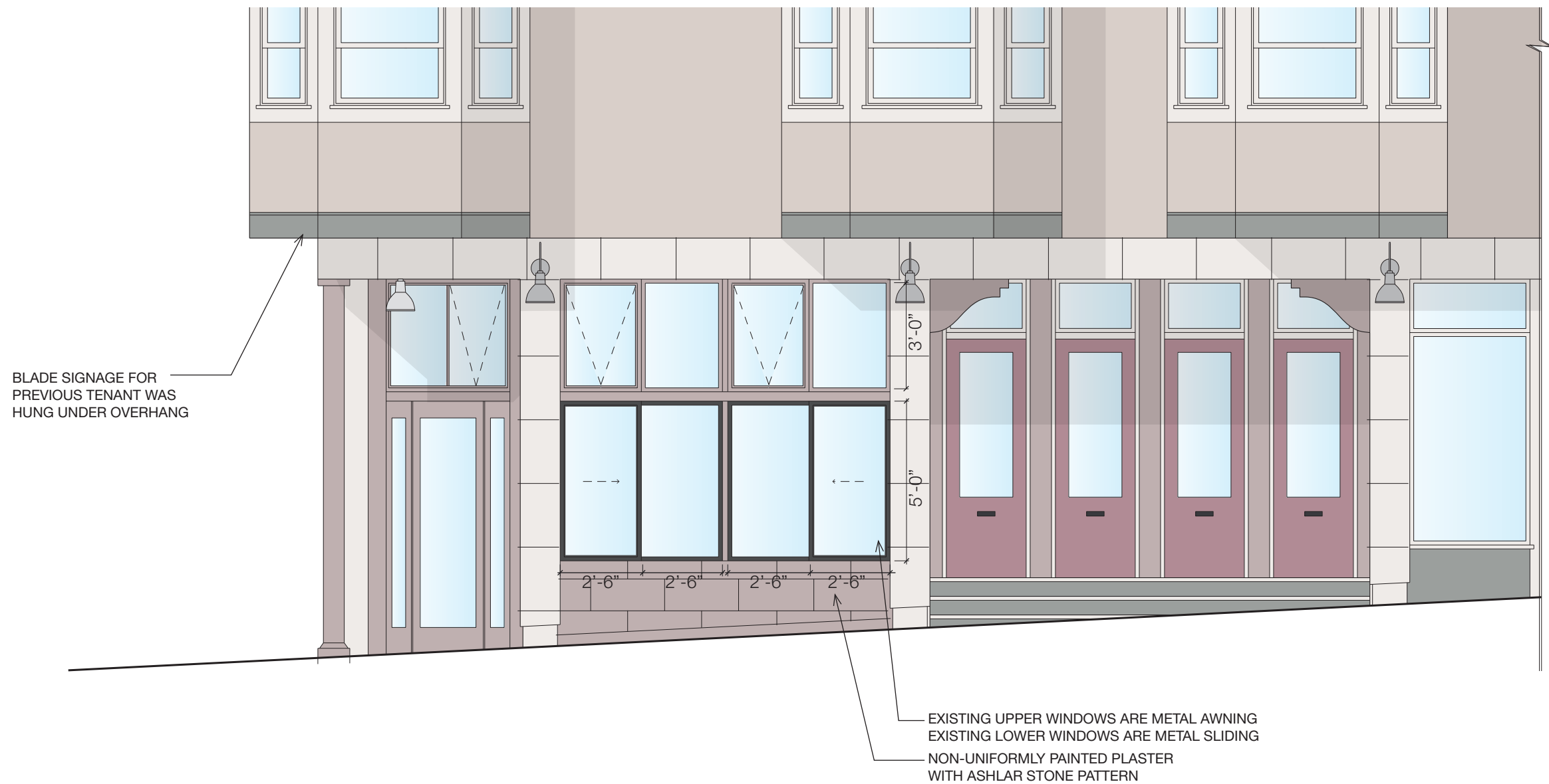
EXISTING EXTERIOR ELEVATION -EAST 1/4" = 1'-0"
