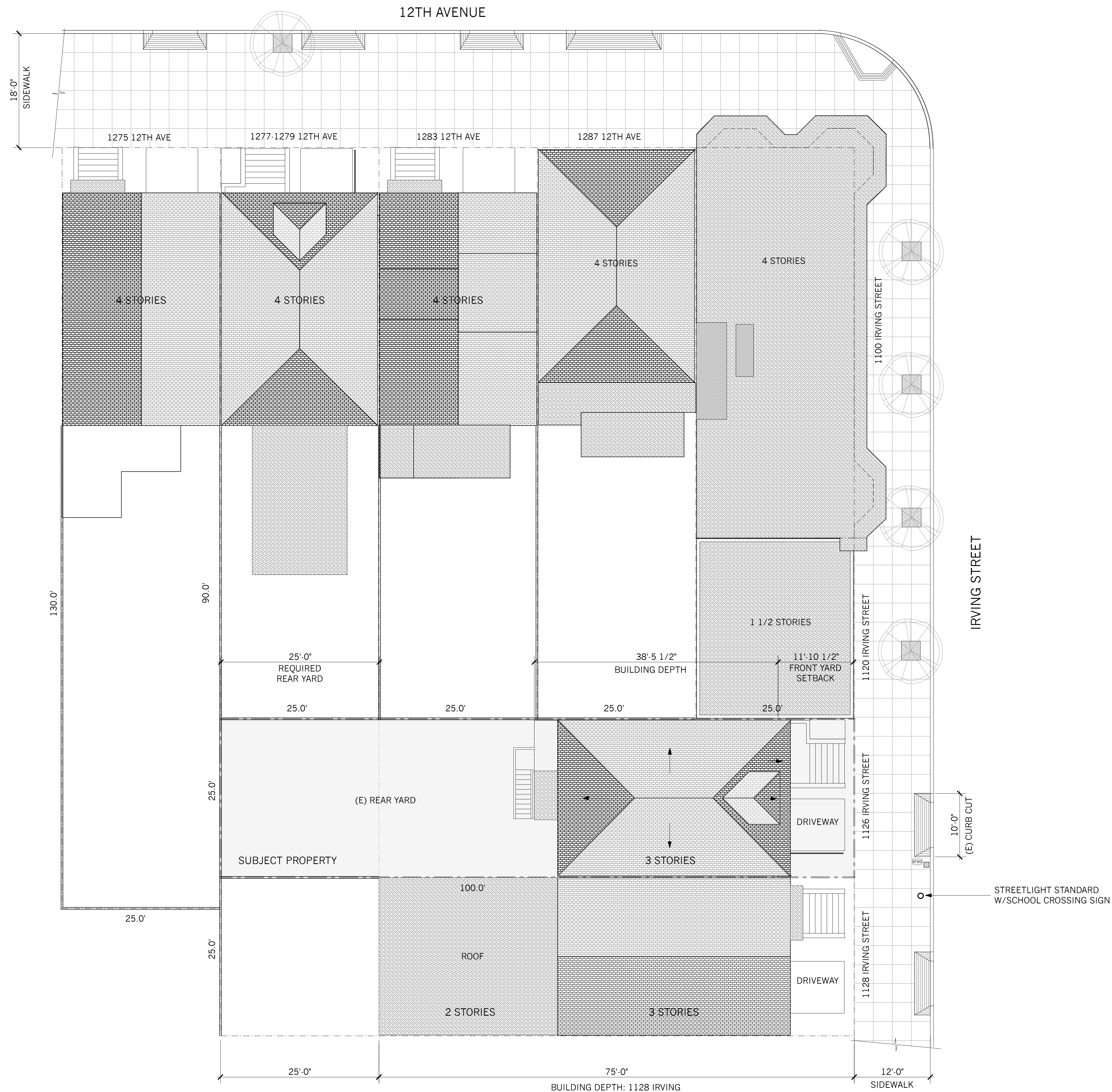
1 EXISTING SITE / ROOF PLAN Scale: 1/8" = 1'-0"
