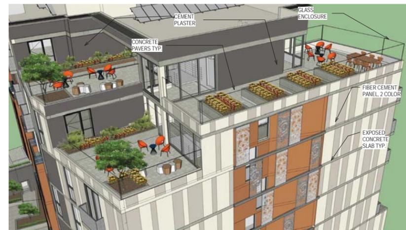
ROOF DECKS 3D MODEL
