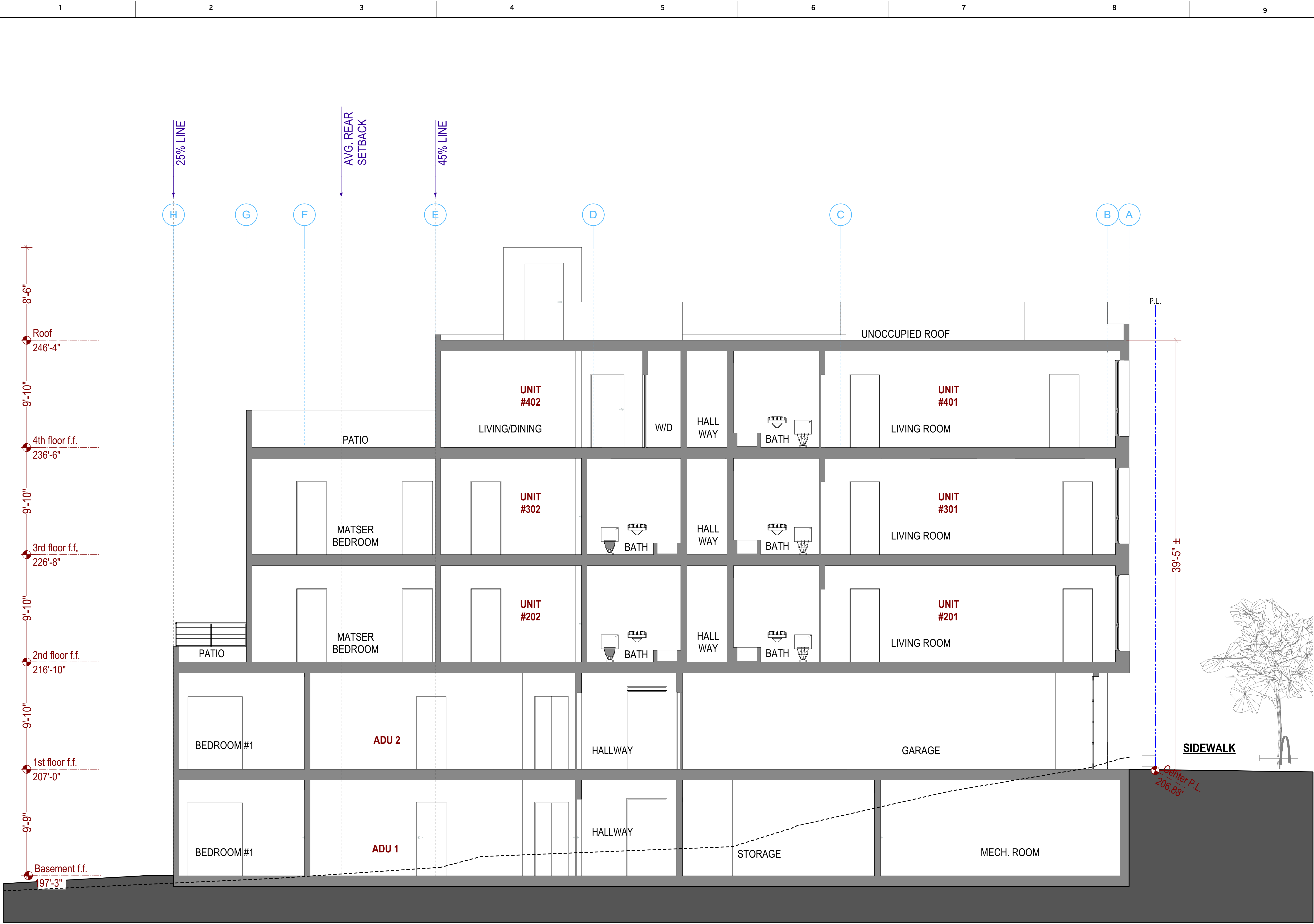
Building Section A-A 1/4" = 1'-0"
