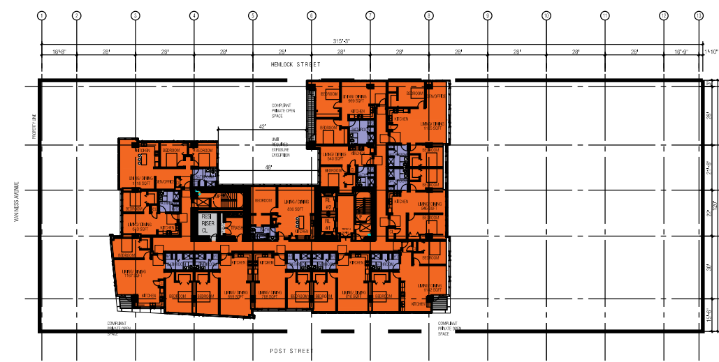
Occupied Floor Area Level 9-13 Total (per floor) - 11827 Residential - 11827 Restrooms (Excluded) - 1248 Bldg Services (Excluded) - 216 1 LEVEL 9-13 SCALE: 1/64" = 1'-0"
