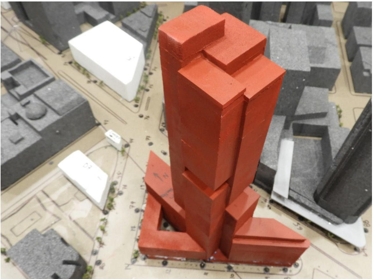
Image 2B: Wind Tunnel Study Model – Existing + Variant Configuration
