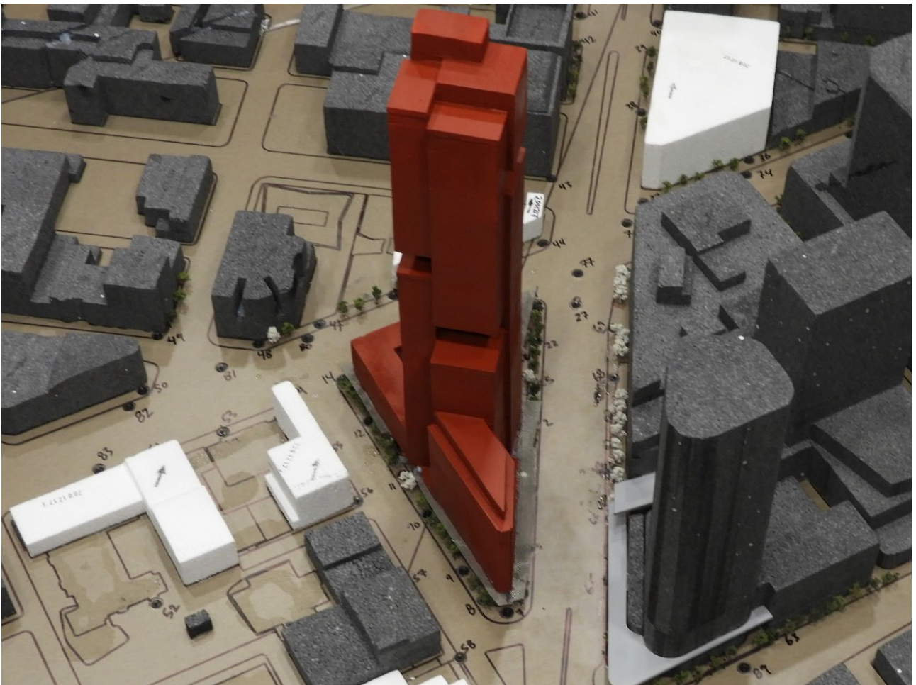
Image 2C: Wind Tunnel Study Model – Existing + Variant + Wind Reduction Features Configuration
