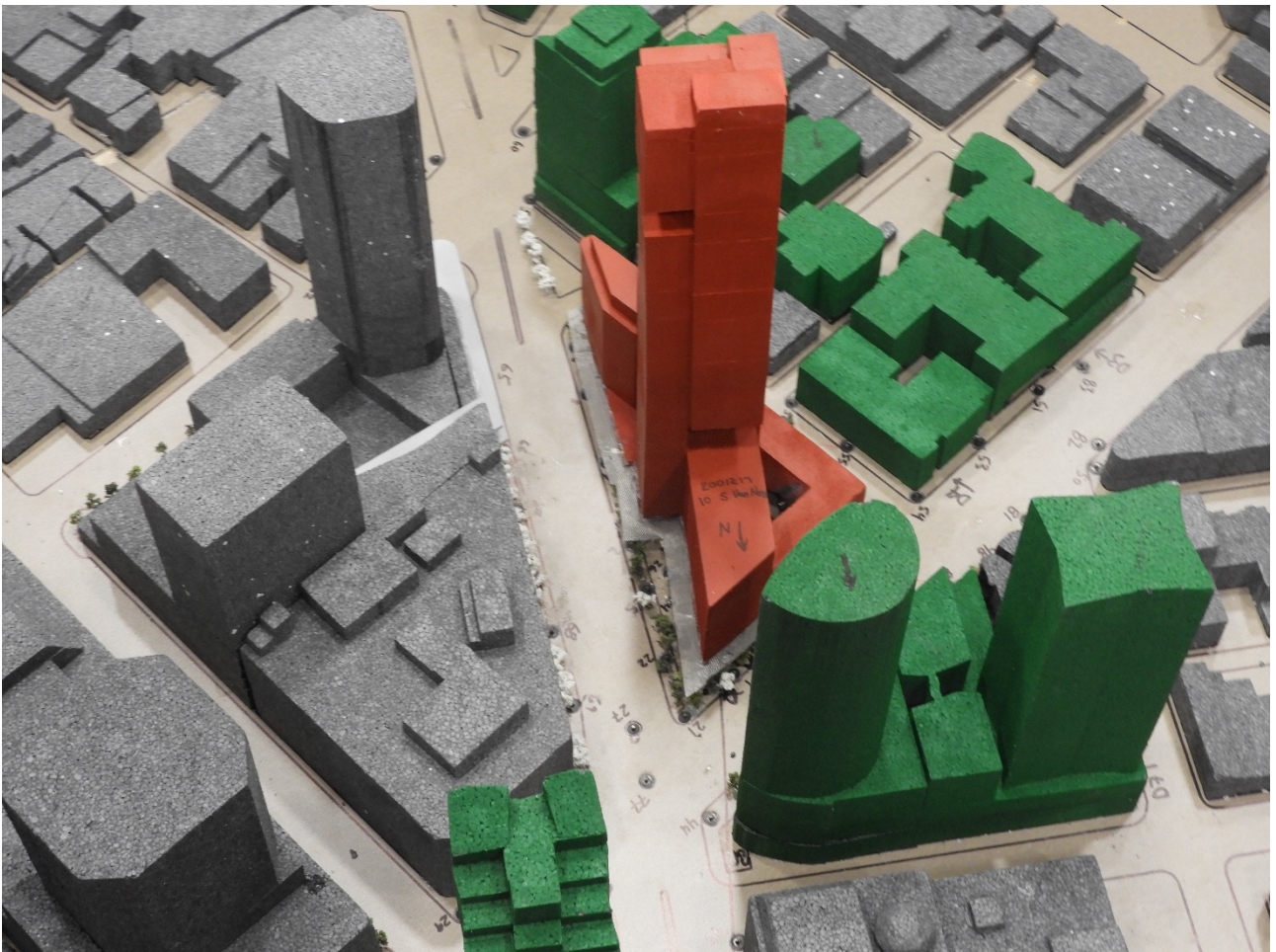
Image 2D: Wind Tunnel Study Model – Variant + Wind Reduction Features + Cumulative Configuration
