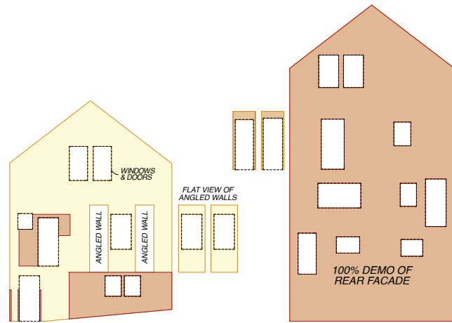
Front Facade Demo Diagram LIGHT GREY = 533 s.f. total original front facade (includes windows & doors) DARK GREY = 103 s.f. total Demolished framing at front facade TOTAL DEMO OF FRONT FACADE = 19.3%
