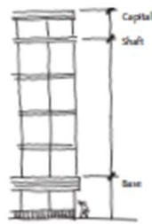
Fig. 56 Base, Shaft, Capital - A Typical San Francisco Building Pattern
