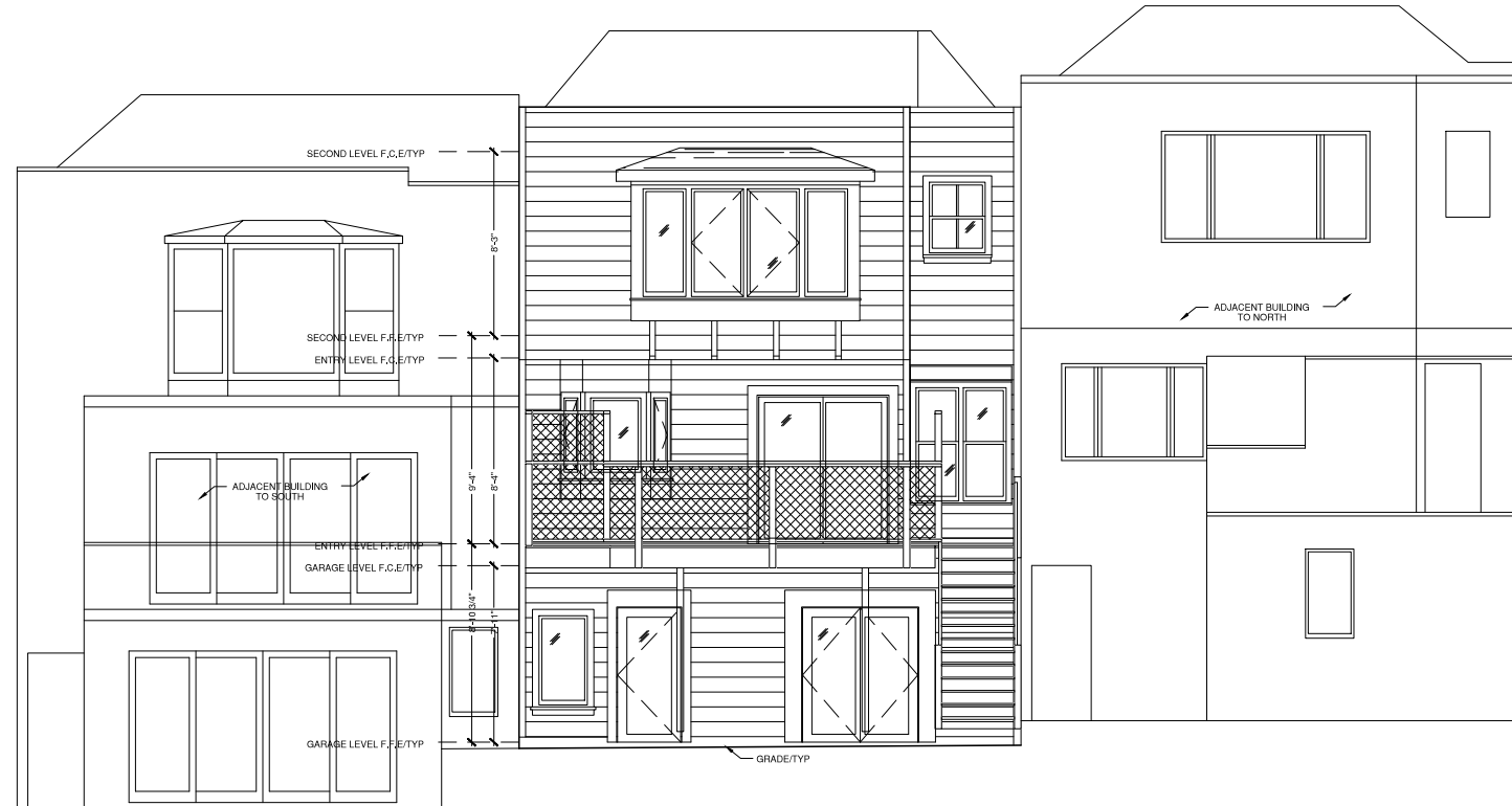
1 EX1.4 EXISTING SOUTH ELEVATION SCALE: 1/4"=1'-0"
