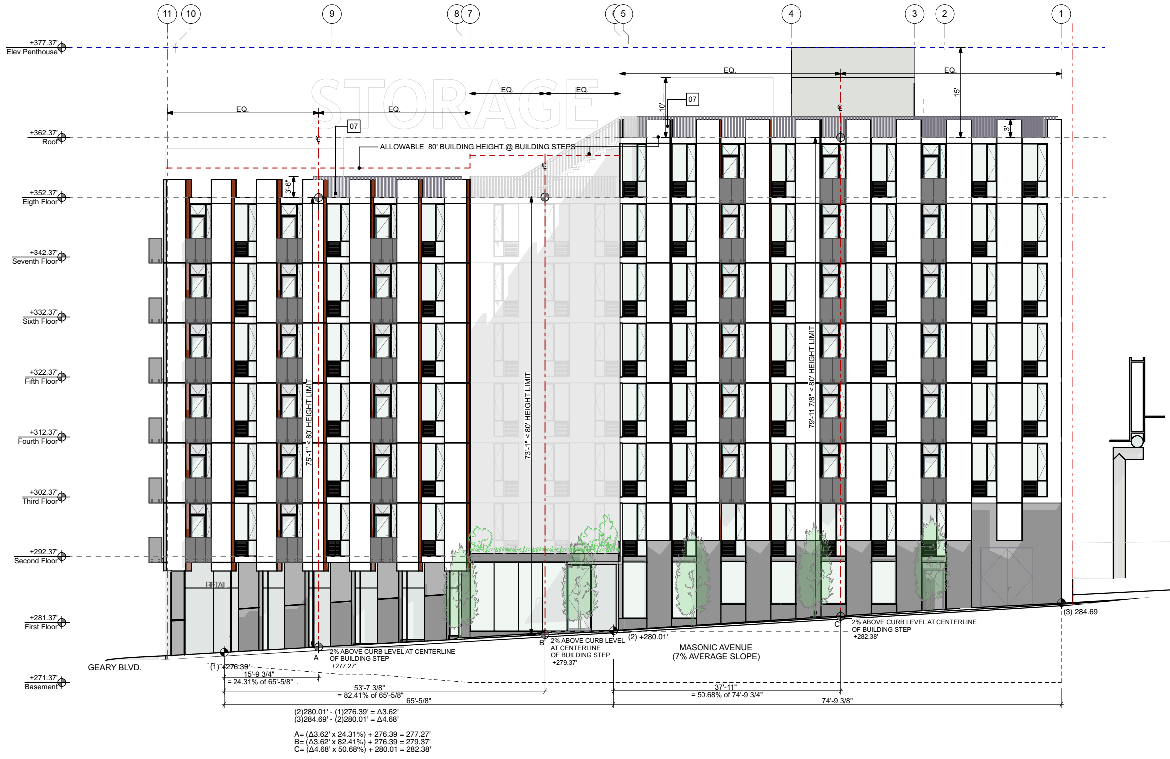
MASONIC AVE (EAST) ELEVATION SCALE: 1/16" = 1'-0"
