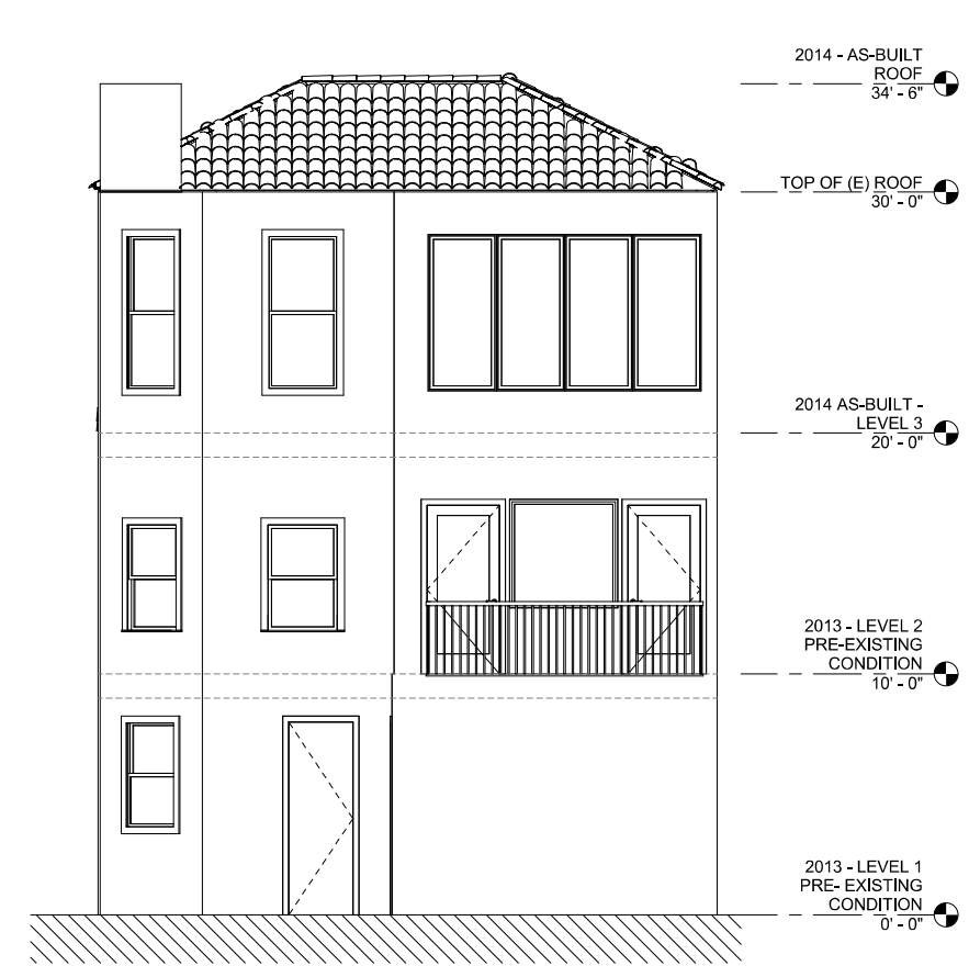
2 2014 - AS-BUILT REAR ELEVATION 1/4" = 1'-0"
