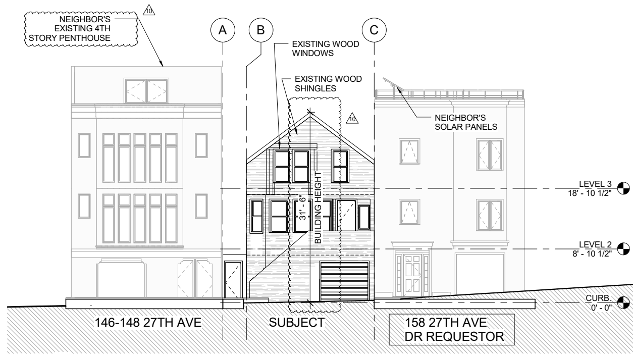
1 EXISTING FRONT ELEVATION - WEST 1/8" = 1'-0"
