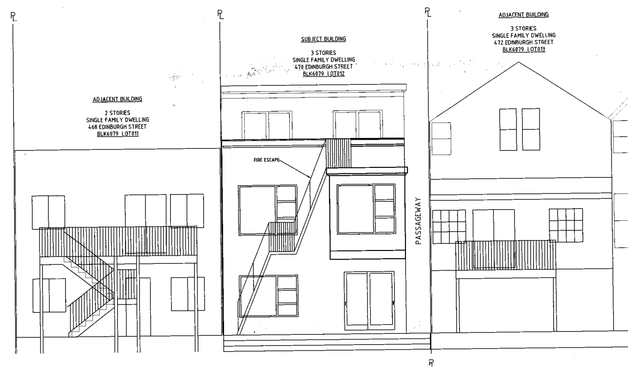
PROPOSED REAR ELEVATION W/ ADJACENT BUILDING ( 3/16" = 1'-0" )
