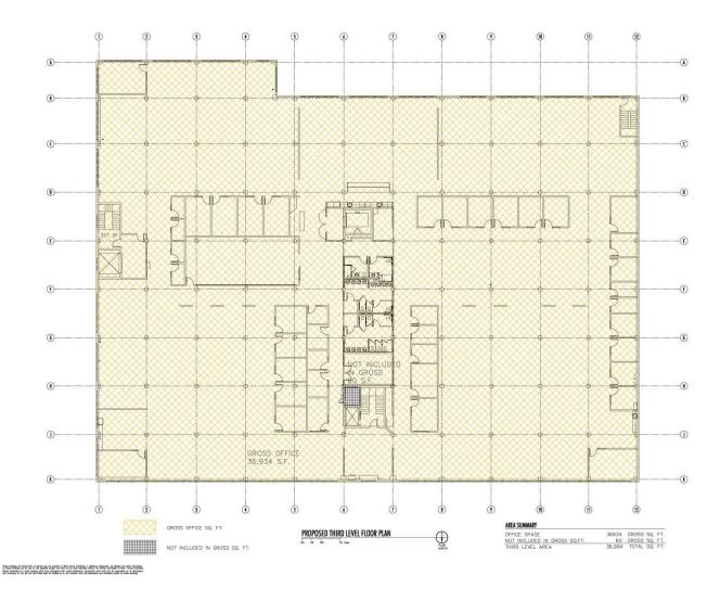
Figure 8 -Proposed Third-Level Floor Plan
