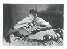
ENGRAVING. Copper-plate and steel-die engraving is a painstaking hand operation requiring years of experience on the artist's part. Few men are engaged in this specialized profession today. ABOVE, the veteran engraver at A. Carlisle & Co., surrounded by an array of cutting implements, engraves a copper diploma plate. BELOW, the steel-die stamping press in operation.
