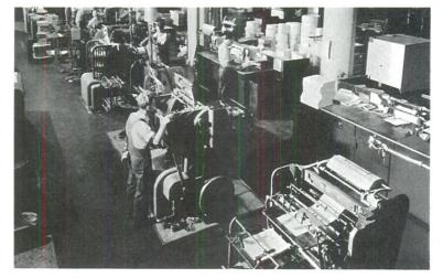
LEFT. Job presses, for all types of small-size, small-run commercial letterpress printing. Plant is equipped with eleven of these presses of various sizes. They handle the bulk of A. Carlisle & Co.'s commercial printing. Typical jobs: letterheads, statements, invoices, and securities. This picture shows the spaciousness of work areas in the plant.
