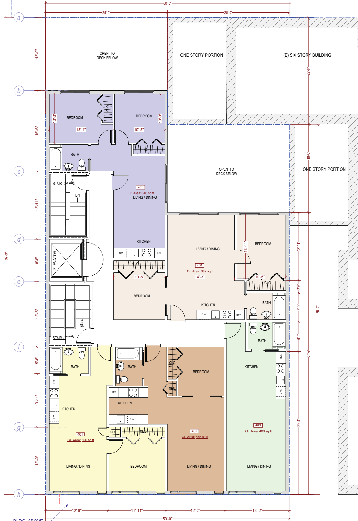
Proposed Fourth Floor Plan 3/16" = 1'-0"
