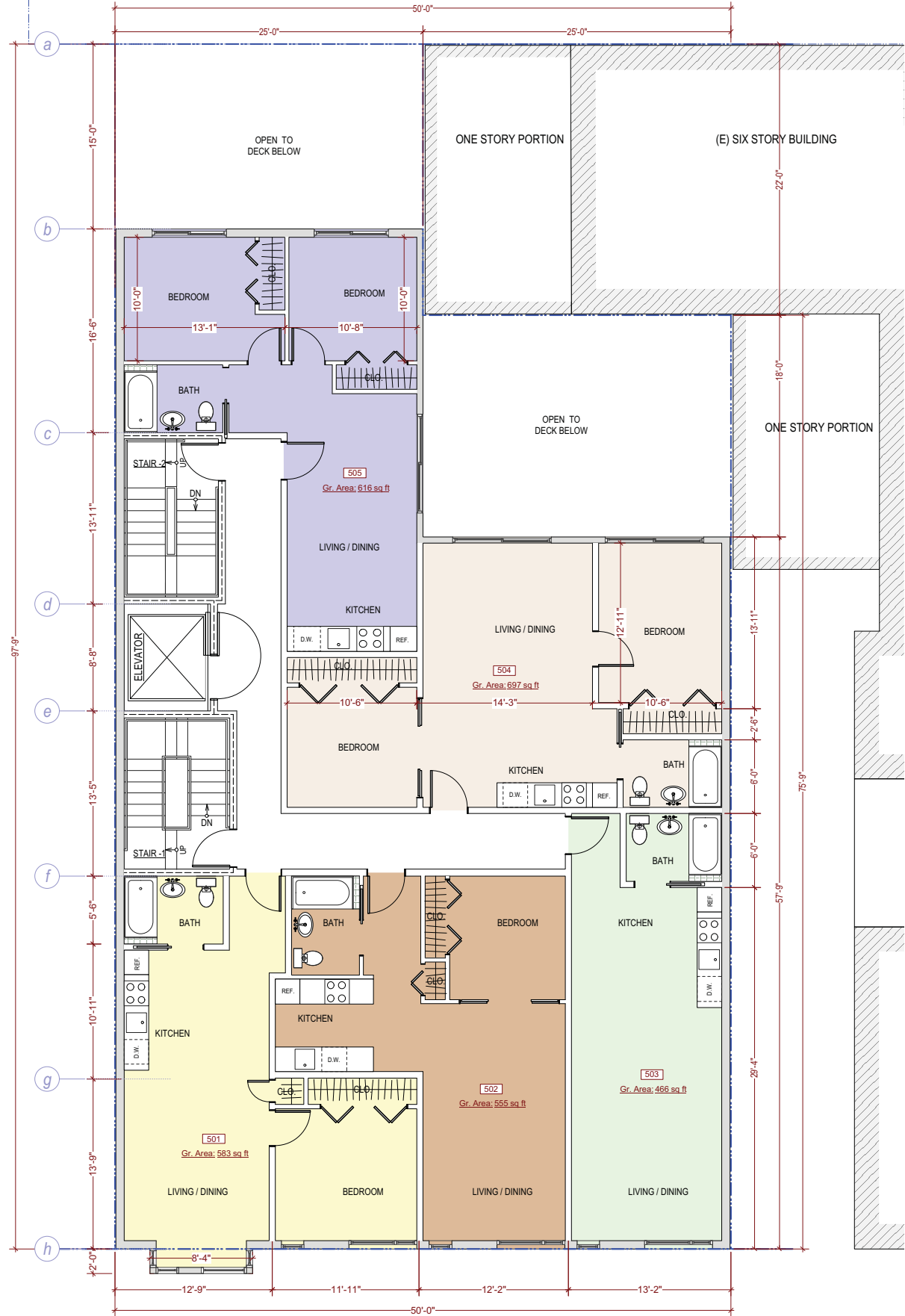
Proposed Fifth Floor Plan 3/16" = 1'-0"
