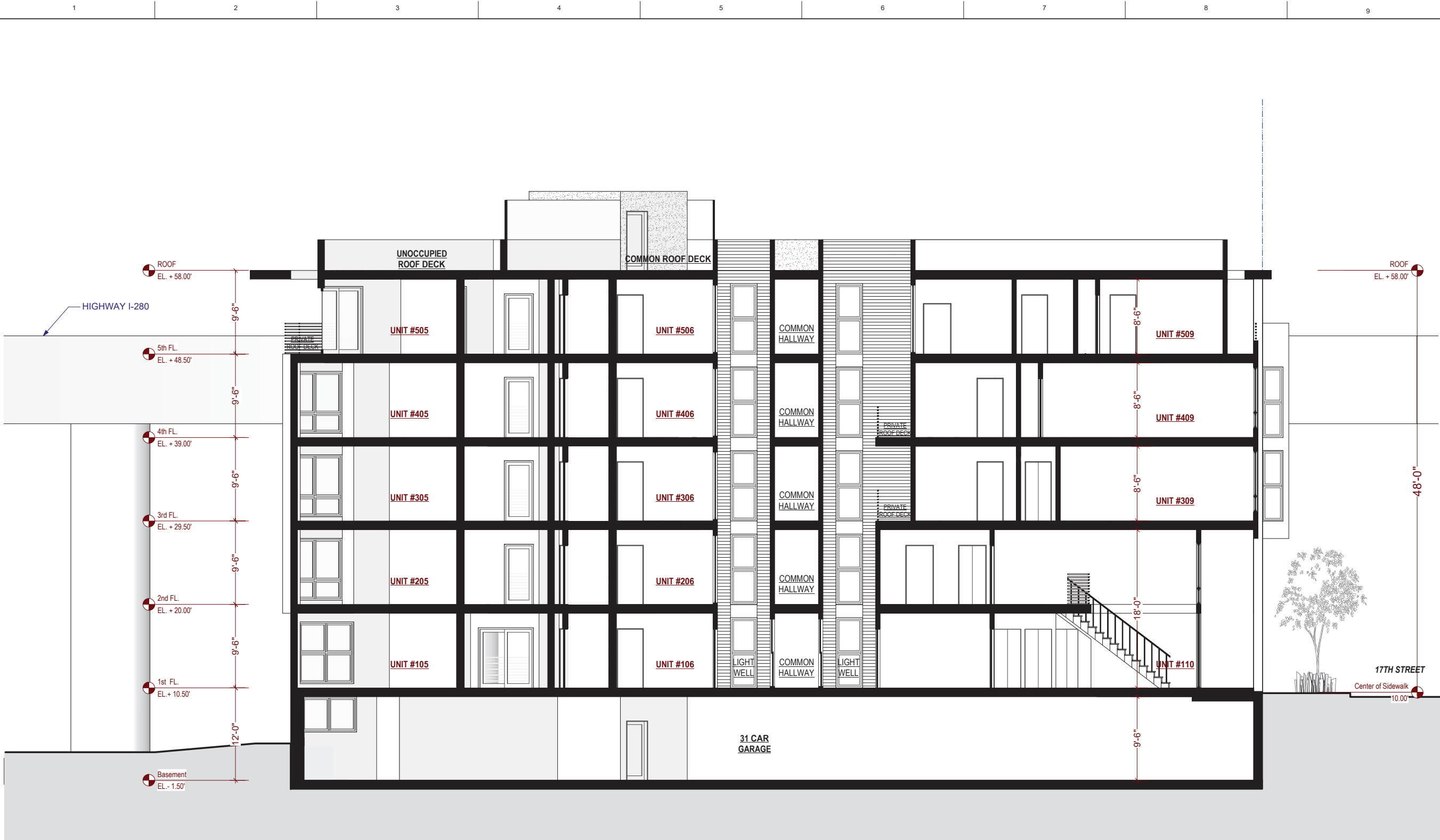
Proposed Section A-A 3/16" = 1'-0"
