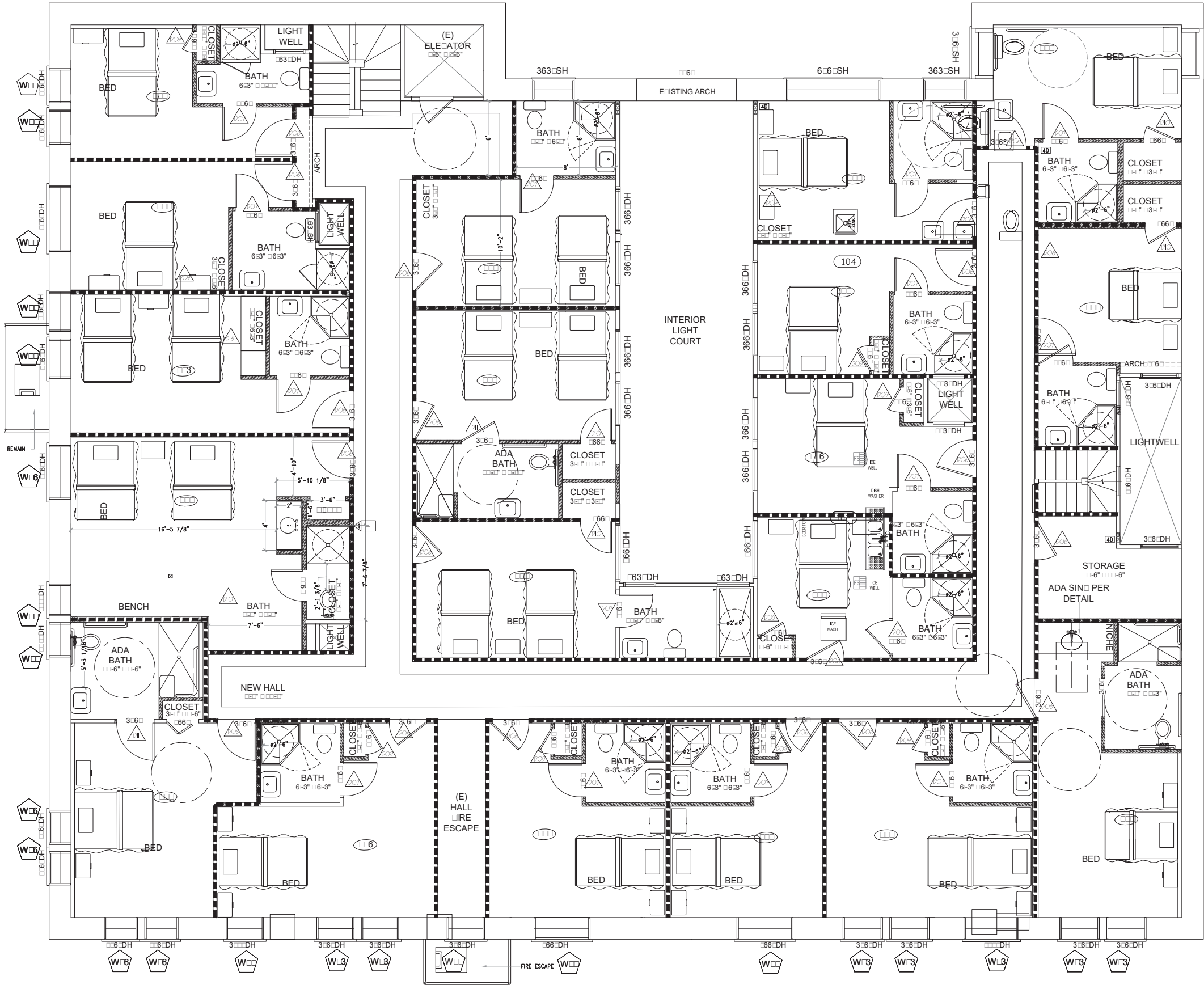
1 NEW 3RD FLOOR PLAN W/WINDOW SCHEDULE W-2 SCALE 1 1/4"=1'-0"
