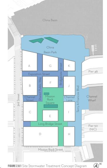
**FIGURE 2.8.1** Site Stormwater Treatment Concept Diagram illustrating watersheds, localized treatment areas, and feature stormwater treatment gardens in the public realm. Refer to Infrastructure Plan for technical requirements.
