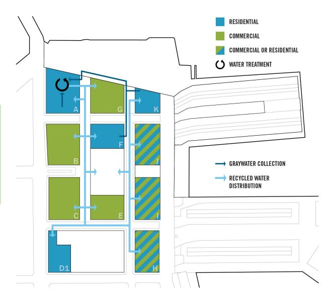
FIGURE A5.2: Graywater collection and recycled water distribution infrastructure
