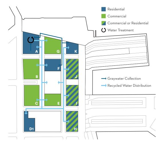
FIGURE 2.4: Graywater Collection and Reclaimed Water Distribution Infrastructure
